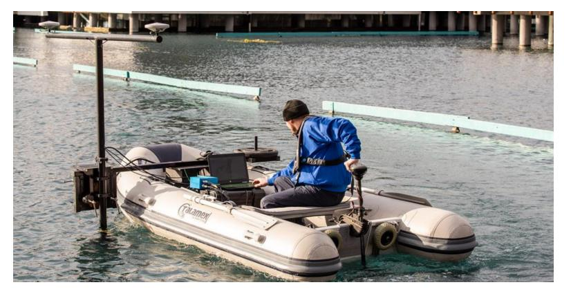
Due local restrictions we used a small electric engine driven 3.5 m (11.5 ft) inflatable boat. The engine used its own battery.
