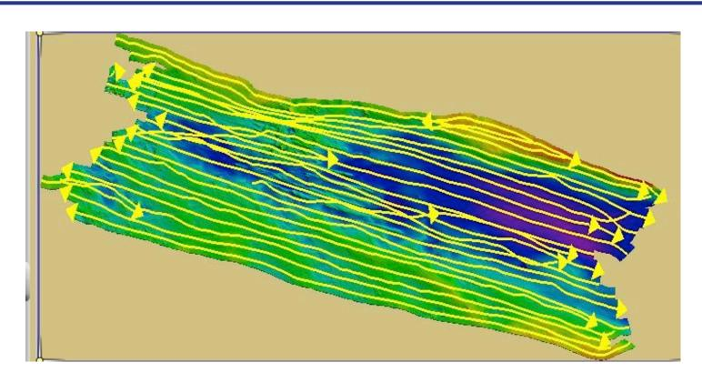
The riverbed structure combined with the very shallow water, and the strong current resulted high turbidity, – what made a nice, parallel navigation impossible.
