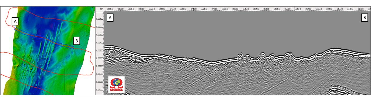
Combination of the A-B geophysical cross-sections with depth (left) and the original seismic (subsurface) dataset (right)
